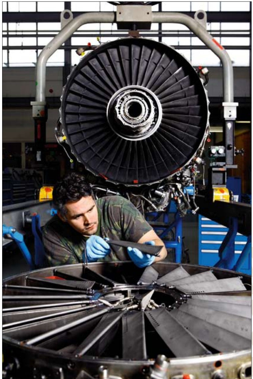
A mechanic inspects a blade of the turbine of the F-100 engine, the engine of the F16 fighter
